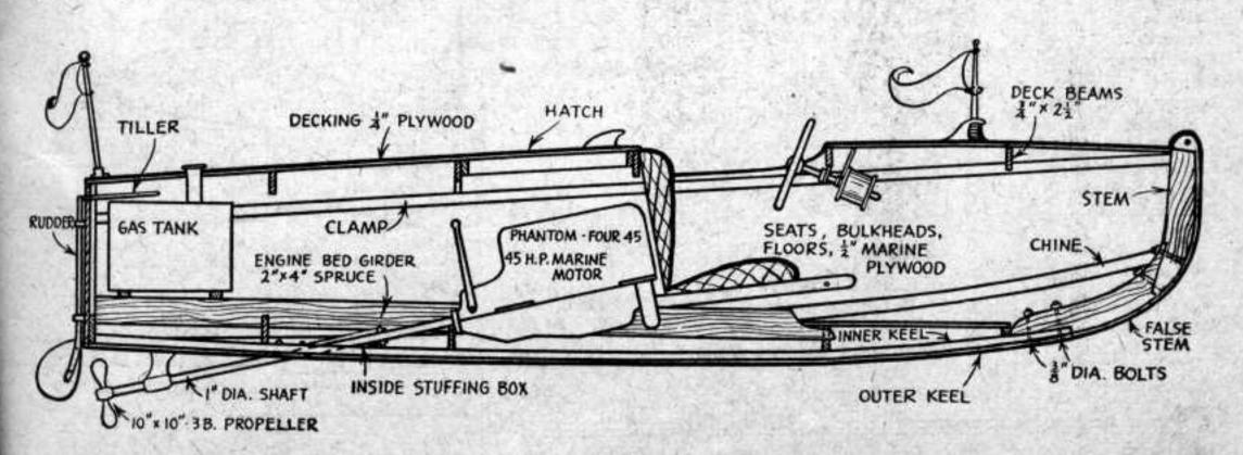
indicated. Notch out form for each frame assembling all parts on form, clamping or nailing wood strips to hold frames in proper alignment, "square" transom with form, and brace securely.
