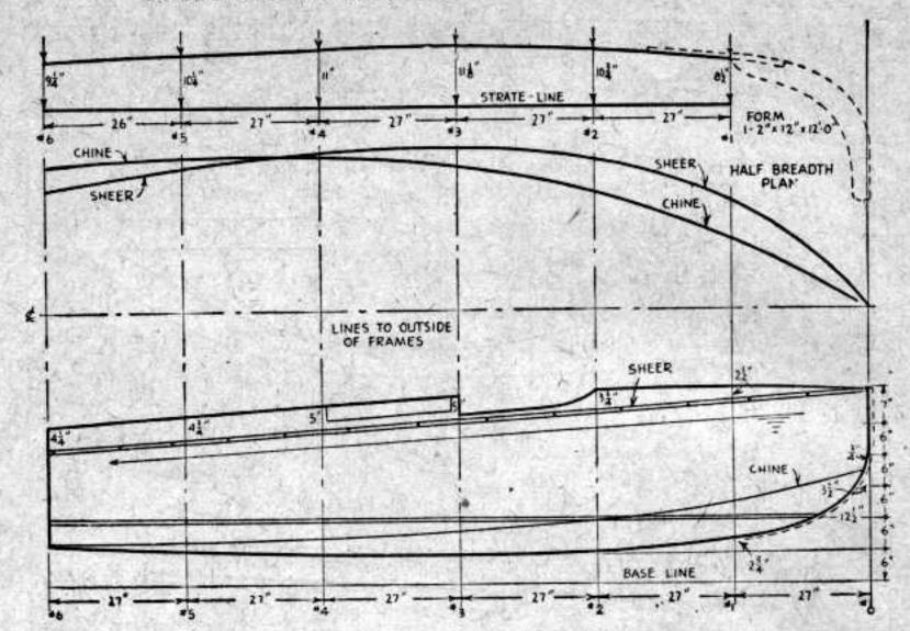
hard service with inboard motors. Fasten battens to frames with 1½" No. 8 F.H. screws, being careful to notch the frame only of the transom and not plywood transom also.
