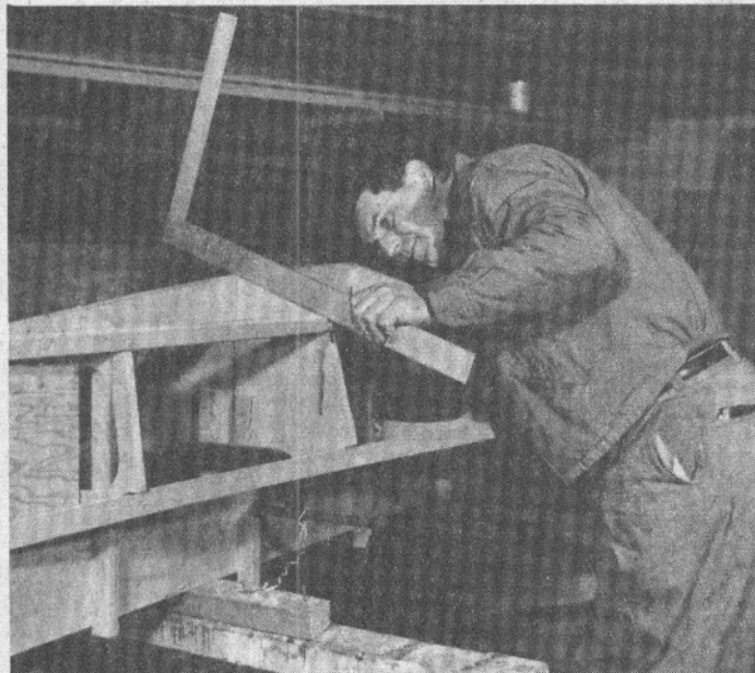
Fig. 2. Check as you go by holding straight edge against keelson, chine strip. Bevel on keelson, chine should conform to straight edge which should slide past frames, just touching.
