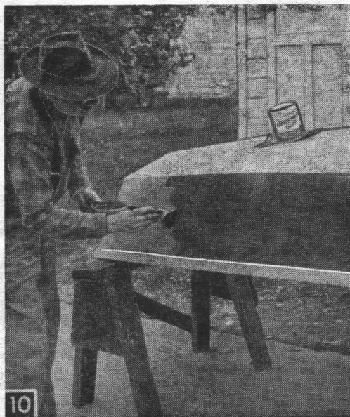
10 Apply generous coating of Elmer's Waterproof Glue to bare plywood in preparation for muslin covering. Stretch muslin tightly over glue, then squeegee flat. When glue is set, but not rock-hard, trim edges with razor blade. Around corners, cut out muslin to prevent overlap as ends are wrapped over edge.
