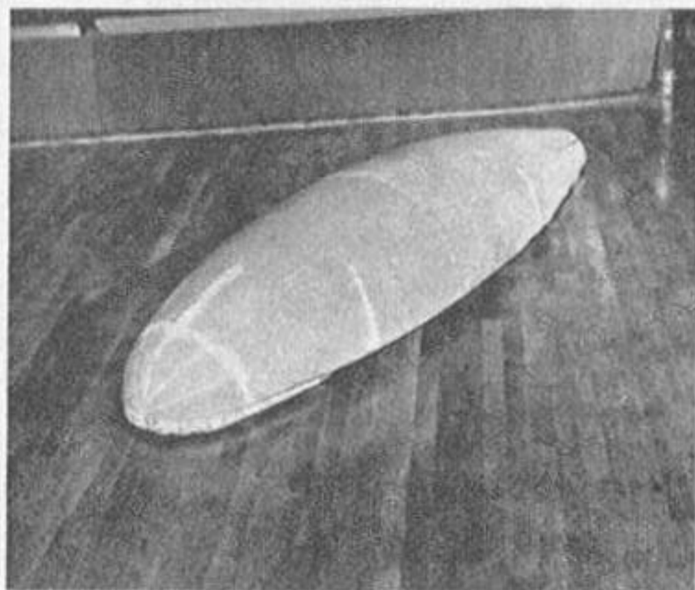
PLYFOAM makes smooth mold, is covered with thin sheet plastic for fiberglass lay-up.
