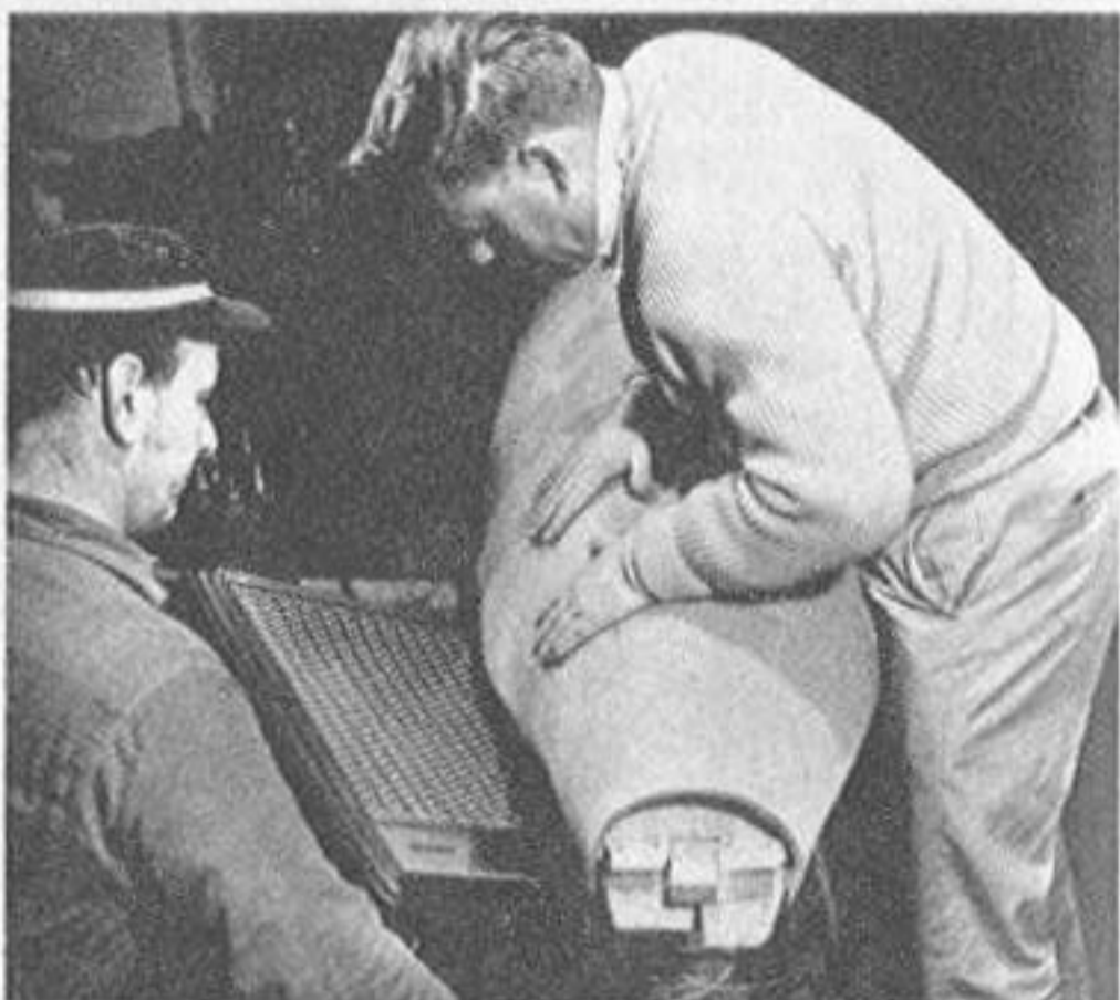
HEATER softens sheet Plyfoam for bending over the ribbands on the basic mold.
