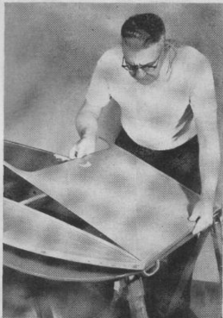
CHECK FIT OF DECK before installing permanently. Make sure screw holes are uniformly spaced and that there are no skips in calking seal. Sand edges flush
