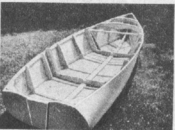
Hull almost finished but mould frames have not been removed. Seats and risers yet to be installed.
