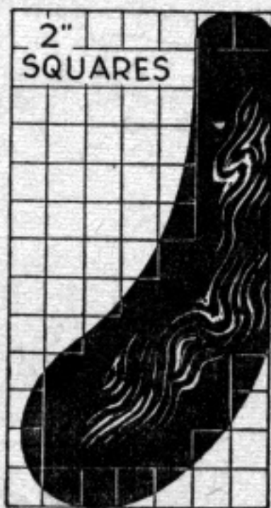
RUDDER \frac{3}{4} " PLYWOOD
