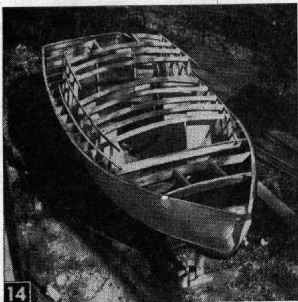
Start of framing for cabin using beams at stations.
