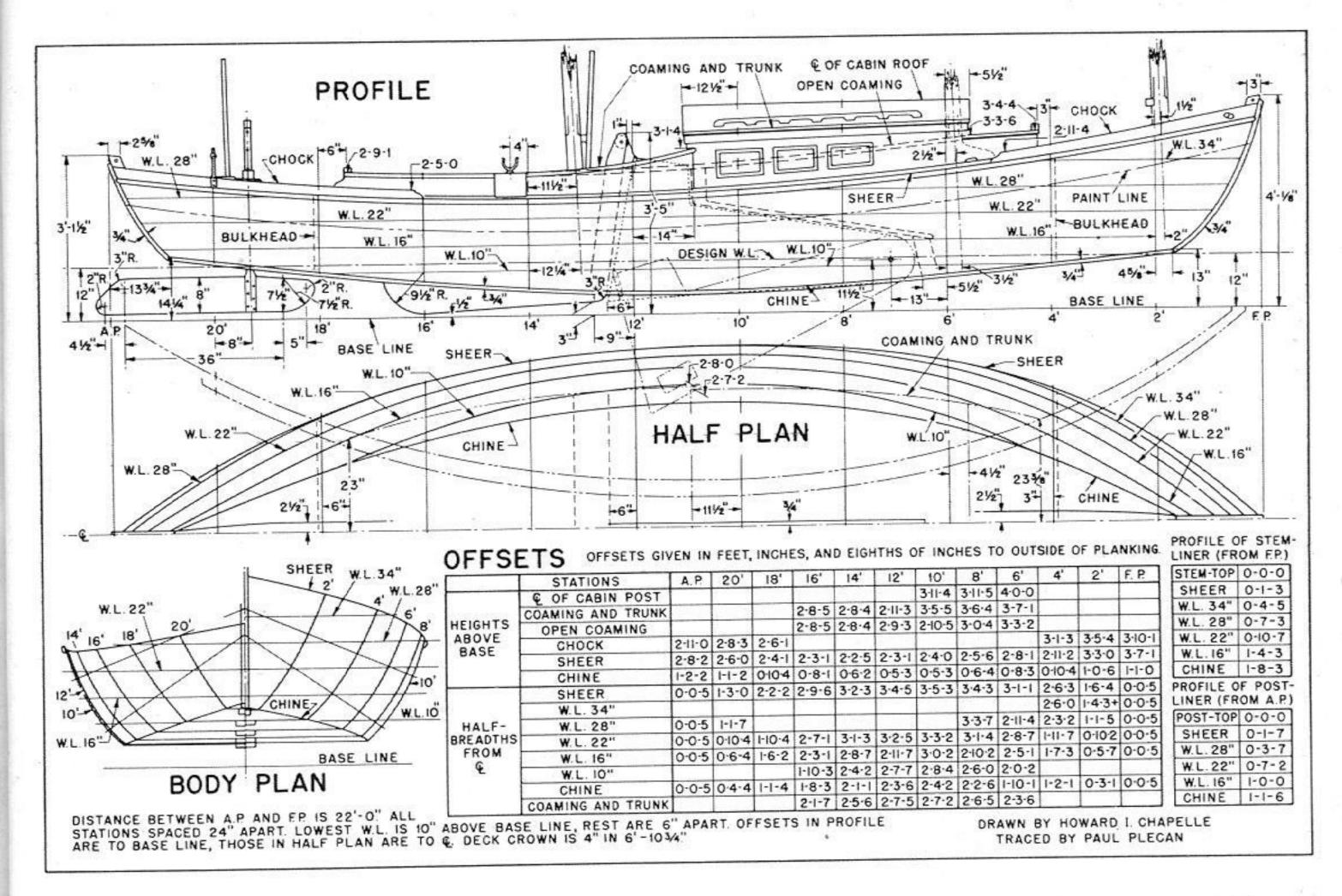
pipe and the mast steps should be placed and secured now. Frames 4 and 18 are formed of bulkheads; these should be gotten out but not assembled; the bottom plank will serve as a floor-timber. There are no floor timbers for frames 2 and 20.
