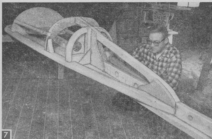
Heavy fuselage framework strengthens main longeron. Photo above taken at forward end looking aft.
