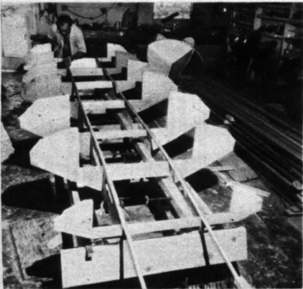
ALL RIBS are in place on the jig with main girders ready to be glued to ribs.
