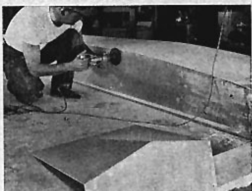
FIBERGLASS HULL before turning it over (Dyneal was used here), then flip the hull and apply the decking
